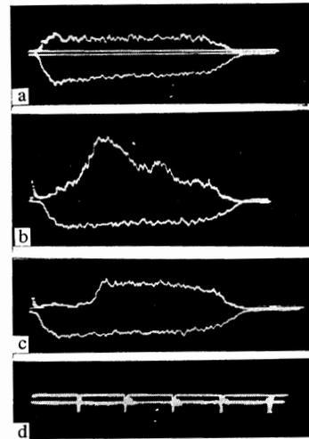
FIG. 3. Oscillograms of the probing signal at initial  $\text{CF}_3\text{I}$  vapor pressure of 40 Torr and wavelengths of 2600 Å (b) and 2850 Å (c); a – time dependence of the EV-45 source itself with a supplementary line; d – timing marks at 100  $\mu\text{sec}$  intervals. The negative pulse is a reference channel signal. The pumping and probing pulses are started simultaneously.
