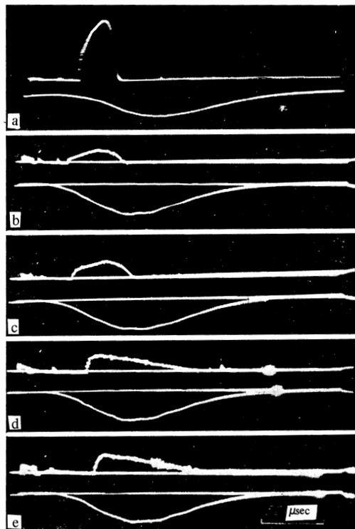
FIG. 5. Oscillograms of  $\text{CF}_3\text{I}$  PDL emission (20 Torr) for various argon pressures: a – 0, b – 55, c – 100, d – 500, e – 700 Torr. In the case of oscillograms b, c, d, and e the sensitivity of the receiver is the same and is lower than in the case of oscillogram a. The second beam recorded the pumping pulse; its maximum corresponds to  $T_{\text{brt}} = 10,300^\circ$ .
