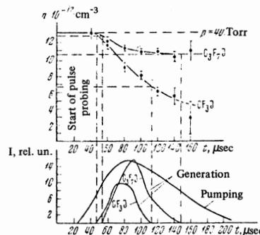
FIG. 7. The function  $\Delta n_{\text{eff}}(t, \lambda_{\text{max}}^0)$  (initial pressure of  $CF_3I$  and  $C_3F_7I$  is 40 Torr,  $\lambda_{\text{max}}^0 \approx 2600 \text{ \AA}$ ).
