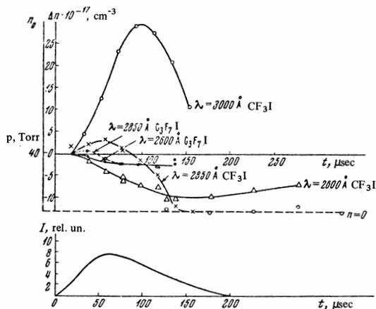
FIG. 2. The function  $\Delta n_{\text{eff}}(t, \lambda)$  for  $\text{CF}_3\text{I}$  and  $\text{C}_3\text{F}_7\text{I}$  at an initial pressure of 40 Torr. (In the computation of  $\Delta n_{\text{eff}}$  it was difficult to take into account the small variation of this quantity in the time interval from 0 to 20  $\mu\text{sec}$ ; it is therefore not reflected in the above curves).
