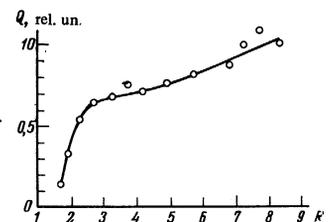
FIG. 2. Dependence of the diamagnetic signal on the effective mirror ratio.  $H_0 = 870$  Oe,  $U_e = 17$  kV,  $I_e = 4$  A.
