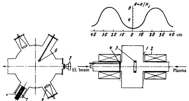
FIG. 1. Diagram of PN-3 installation: 1-vacuum chamber, 2-magnetic-field coil, 3-diamagnetic probe, 4-teflon ring, 5-photographic camera, 6-aluminum target, 7-lead collimator, 8-copper filter, 9-horn antenna. On the right is shown a plot of the magnetic field.
