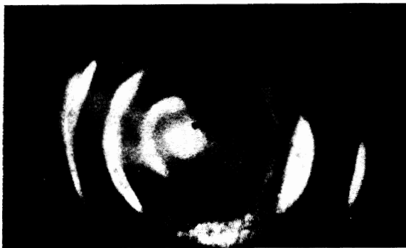
FIG. 1. Radiation pattern of anti-Stokes components of SRS in aragonite, observed at \psi = 0.58 \times 10^{-2} rad. To the left of the laser spot are the half-rings of the fundamental emission of the four anti-Stokes components; to the right appears the supplementary emission of the same components.
