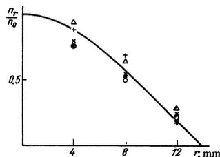
FIG. 2. Radial distribution of charged particle density in helium ( $p = 0.5$  mm Hg,  $i = 25$  mA): (●)  $H = 0$ , (×)  $H = 10$  Oe, (○)  $H = 100$  Oe, (Δ)  $H = 300$  Oe, (+)  $H = 500$  Oe.
