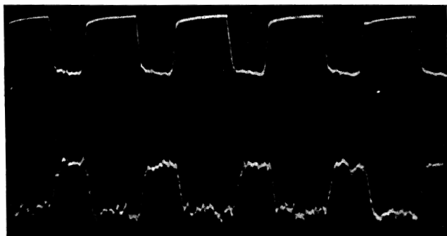
FIG. 2. Oscillograms of the pulse amplitude proportional to P (upper trace) and of the pulse amplitude proportional to \Delta I_{sp} (lower trace).
