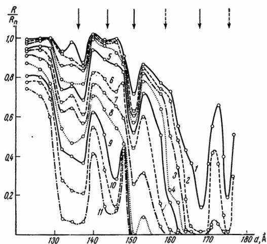
FIG. 1. Relative resistance of tin films as a function of the thickness. Temperature ( $^{\circ}$ K): 1—4.041, 2—4.038, 3—4.035, 4—4.031, 5—4.026, 6—4.022, 7—4.016, 8—4.010, 9—4.002, 10—3.996, 11—3.992.
