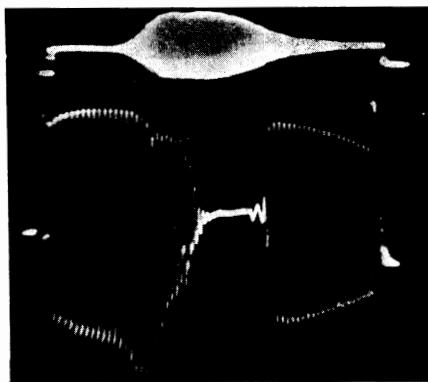
FIG. 1. Oscillogram showing the effect of rf stabilization.  $B = 1.2$   $B_C$ ,  $I_0 \approx 30$  mA, sample  $2 \times 2 \times 5$  mm.
