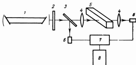
FIG. 2. Block diagram of the apparatus: 1) He-Ne laser, 2) filter, 3) semitransparent mirror, 4) long-focus lens, 5) semiconductor sample, 6) radiation detector, 7) differential amplifier, 8) oscilloscope.
