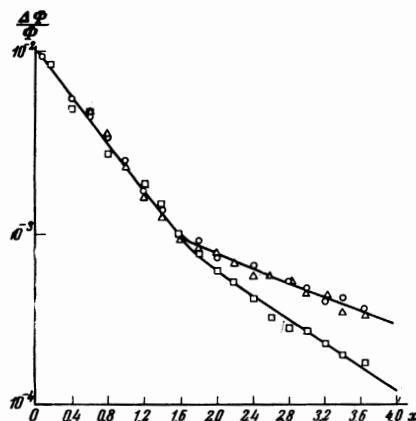
FIG. 3. Absorption curve of light along the axis of the semiconductor sample with dimensions  $2 \times 2 \times 5$  mm ( $s = 1600 \text{ cm sec}^{-1}$ ):  $\circ$ )  $B = 0.9 B_c$ ;  $\square$ )  $B = 1.2 B_c, I_1 = 0$ ;  $\Delta$ )  $B = 1.2 B_c, I_1 = 2I_0$ .
