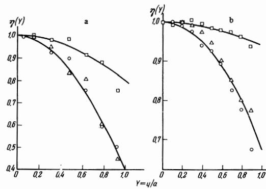
FIG. 4. Curve showing the absorption of light in the direction transverse to the sample: a) Sample with dimensions a)  $2 \times 2 \times 5$  mm,  $s = 1600 \text{ cm sec}^{-1}$ , b)  $1.5 \times 1.5 \times 5$  mm,  $s = 800 \text{ cm sec}^{-1}$ . The notation on the experimental points is as in Fig. 3.
