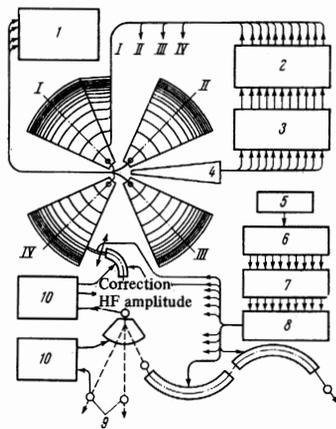
FIG. 2. Block diagram of control system for monoenergetic cyclotron: 1—nuclear field stabilizers, 2—regulated sources of supply for the correcting windings, 3—system for logical processing of the signals from the  $\varphi_n$  pickups, 4— $\varphi_n$  pickups, 5—operator, 6—regime coder, 7—programmer-universal computer, 8—code-analog converter, 9—beam coordinate pickups, 10—analog correction system.
