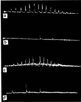
FIG. 2. Oscillograms of generator pulses and pulses that passed through the electro-optical shutter (oscillogram sweep duration was 300 nsec): a – periodic generator pulse sequence at the input to the electro-optical shutter; b – single pulse at shutter output; c – sequence of pulses separated by shutter; d – group of pulses at shutter output.
