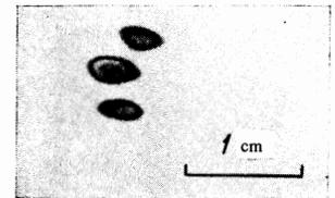
FIG. 6. Photograph of radiation trace on film placed at a distance of 25 m from the amplifier output.
