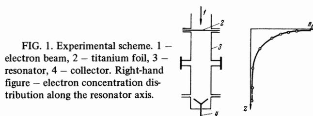
FIG. 1. Experimental scheme. 1 - electron beam, 2 - titanium foil, 3 - resonator, 4 - collector. Right-hand figure - electron concentration distribution along the resonator axis.
