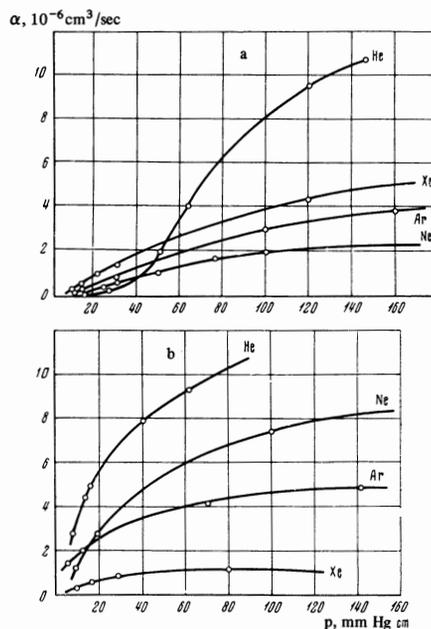
FIG. 3. Recombination coefficients for plasmas produced by (a) a direct discharge and (b) an electron beam.
