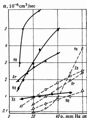
FIG. 2. Recombination coefficient in inert-gas plasmas produced by a direct discharge (dashed curves) and by an electron beam (solid curves).
