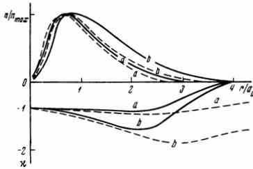
FIG. 2. Reduced density and potential perturbations: (a) for  $x = 0.5$  and (b) for  $x = 1$ . The continuous curve represents the case of zero perturbations and  $\varphi$  for  $\rho = 4$ ; the dashed curve represents  $\rho = 10$ , when there is no boundary effect;  $\kappa = (\varphi/f)/|(\varphi/f)_0|$ .
