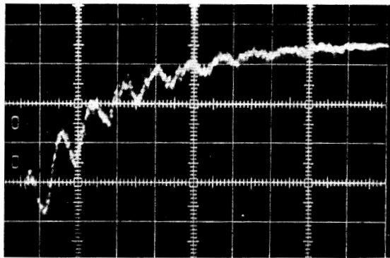
FIG. 2. Oscillogram of the oscillations of the intensity of the afterglow in helium plasma upon cooling of the discharge tube to 4°K (4650 Å band).  $N = 3 \times 10^{17} \text{ cm}^{-3}$ , radius of retort,  $R = 2 \text{ cm}$ ,  $\tau = 5 \mu\text{sec}$  (along ordinate: intensity in arbitrary units, scale along the time axis, one unit corresponds to 200  $\mu\text{sec}$ ; O — start of sweep).
