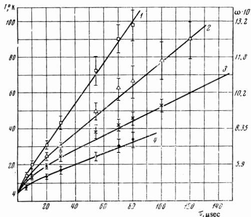
FIG. 5. Dependence of the mean gas temperature on the pulse length  $\tau$  for a current of  $i = 2.3$  A. Curves 1 – 4 correspond to the same gas densities as in Fig. 4.
