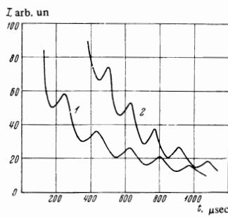
FIG. 3. Oscillations of the intensity of the afterglow ( $\lambda = 4471 \text{ \AA}$ ) for different currents. Cooling of the discharge tube to 4°K,  $\tau = 5 \mu\text{sec}$ ,  $R = 2 \text{ cm}$ ,  $N = 9 \times 10^{17} \text{ cm}^{-3}$  ( $p = 25 \text{ mm Hg}$ ); curve 1 —  $i = 1 \text{ A}$ , 2 —  $i = 2.3 \text{ A}$ .
