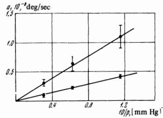
FIG. 7. Dependence of the coefficient  $a_1$  on the reduced pressure (density) of helium for different currents: 1 –  $i = 2.3$  A,  $a_1 p = (9.5 \pm 2) \times 10^6 \text{ deg-sec}^{-1} \text{ mm Hg}$ ; 2 –  $i = 1$  A,  $a_1 p = (3.6 \pm 0.2) \times 10^6 \text{ deg-sec}^{-1} \text{ mm Hg}$ .
