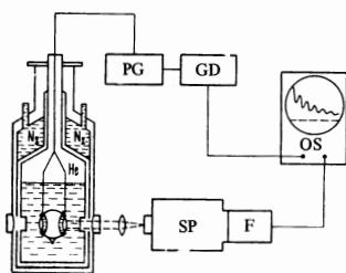
FIG. 1. Schematic drawing of experiment: PG — high-frequency pulse generator; GD — generator of delayed pulses, G5-4B; OS — S1-8 oscillosograph; SP — spectrograph DFS-8, F — photomultiplier FÉU-64 with cathode follower.
