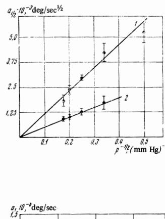
FIG. 6. Dependence of the coefficient  $a_{1/2}$  on the reduced pressure (density) of helium for different currents: 1 –  $i = 2.3$  A,  $a_{1/2}\sqrt{p} = (11.6 \pm 1.8) \times 10^3 \text{ deg-sec}^{-1/2}(\text{mm Hg})^{1/2}$ ; 2 –  $i = 1$  A,  $a_{1/2}\sqrt{p} = (5.2 \pm 1) \times 10^3 \text{ deg-sec}^{-1/2}(\text{mm Hg})^{1/2}$ .
