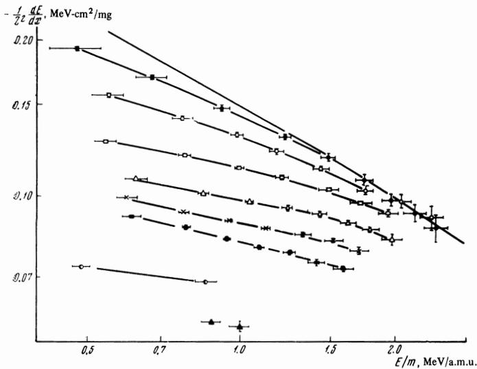
FIG. 1. Stopping ability of Ar as a function of the ion energy: ●—Li, ○—Be, □—B, △—C, ×—N, ■—O, ●—Na, ▲—Al.
