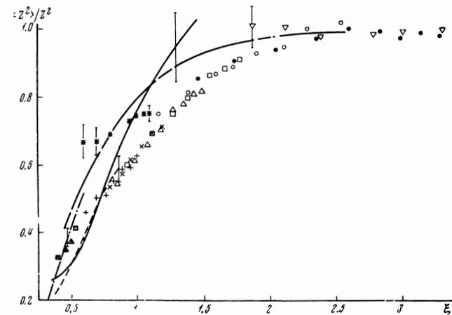
FIG. 2. Dependence of the mean-square charge on the ion velocity. Present work: ●—Li, ○—Be, □—B, △—C, ×—N, +—O, ■—Na, ▲—Al; Ref. 2: ▽—C, \*—Ar; Ref. 5: solid curve—Li, dashed—B, dash-dot—N; Ref. 14: long dashes—deceleration in Al.
