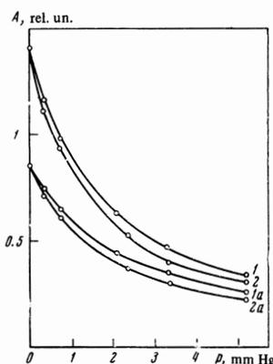
FIG. 8. Dependence of the scintillation pulse amplitude  $A$  on the oxygen-impurity pressure  $p$ . Ionization with  $\alpha$ -particles, pressure of xenon 10 atm. Curves 1 and 1a were obtained at distance of 22 mm from the  $\alpha$  source to the chamber window; 2 and 2a - 46 mm. Curves 1 and 2 were plotted without a field, curves 1a and 2a in the presence of an electric field ensuring a maximum decrease of the amplitude.
