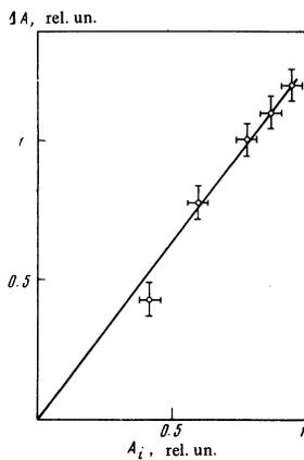
FIG. 2. Decrease of scintillation amplitude  $\Delta A$  vs. amplitude of ionization pulse  $A_i$ . Ionization by  $\alpha$ -particles, xenon density  $0.66 \text{ g/cm}^3$ .
