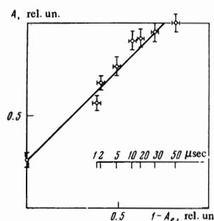
FIG. 7. Dependence of the scintillation amplitude  $A$  on the decrease of the electroluminescence amplitude. The points were obtained for different instants of time following the ionization of xenon by x-rays.
