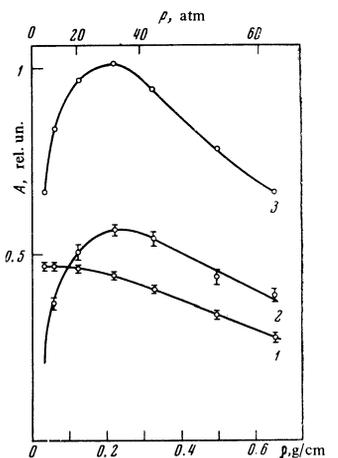
FIG. 4. Dependence of the scintillation amplitude A on the xenon density  $\rho$ . Ionization with  $\alpha$ -particles: 1—the scintillation amplitude component independent of the field, 2—the field-dependent component of the scintillation amplitude, 3—total scintillation amplitude.
