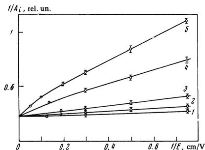
FIG. 3. Dependence of the reciprocal amplitude of the ionization pulse  $1/A_i$  on the reciprocal electric field intensity  $1/E$  in xenon ionized by  $\alpha$ -particles. The curves are obtained at xenon densities: 1—0.125, 2—0.205, 3—0.325, 4—0.495, 5— $0.655 \text{ g/cm}^3$ .
