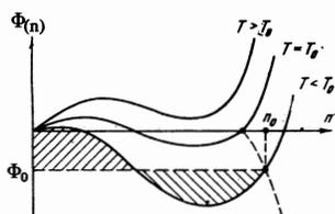
FIG. 2. Schematic graph of the relation  $\Phi = \Phi(n)$  for different temperatures. For a globule having a continuous density distribution,  $\Phi_0 = \Phi(n_0)$  is found from the condition  $\int_0^{n_0} (\Phi - \Phi_0) dn = 0$ . The temperature  $T_0$  at which appearance of such a globule becomes possible corresponds to the values  $\Phi_0 = 0$ .
