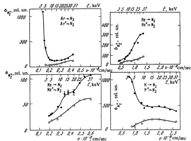
FIG. 2. Plots of the effective cross sections for the production of N<sub>2</sub><sup>+</sup> ions against the velocity of the ions and atoms of hydrogen, neon, and argon. ●—positive ions, ○—neutral atoms.
