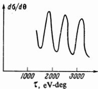
FIG. 1. Differential cross section of scattering of  $\text{He}^+$  by Ne at  $E_{\text{lab}} = 400$  eV and  $F_2/F_1 = 0.14$ . The absolute scale is arbitrary.
