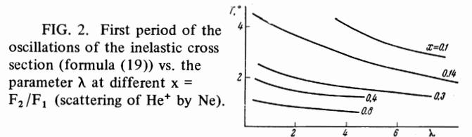
FIG. 2. First period of the oscillations of the inelastic cross section (formula (19)) vs. the parameter  $\lambda$  at different  $x = F_2/F_1$  (scattering of  $\text{He}^+$  by Ne).
