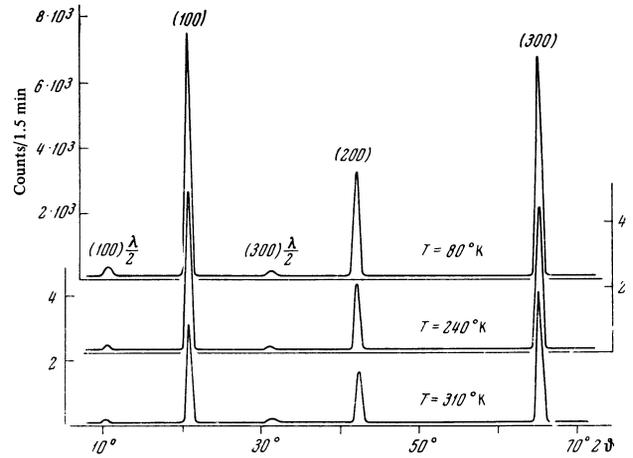
FIG. 3. Neutron diffraction patterns of  $Gd^{160}$ , corresponding to the direction [001] in the reciprocal lattice at 80, 240, and 310° K.
