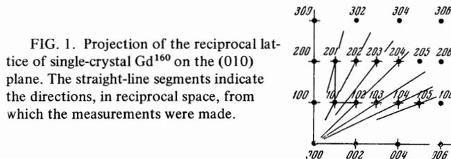
FIG. 1. Projection of the reciprocal lattice of single-crystal  $Gd^{160}$  on the (010) plane. The straight-line segments indicate the directions, in reciprocal space, from which the measurements were made.
