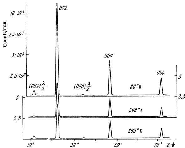
FIG. 2. Neutron diffraction patterns of  $Gd^{160}$ , corresponding to the direction [100] in the reciprocal lattice, at 80, 240, and 295° K.
