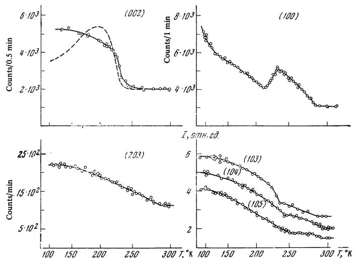
FIG. 4. Temperature dependence of the peak values of the diffraction maxima for  $Gd^{160}$ . Dashed curve — data of [3].
