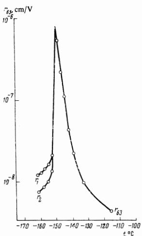
FIG. 1. Electro-optical coefficients  $r_i$  as functions of temperature for the KDP crystal.  $r_{63}$  — at  $T > T_c$ ;  $r_1, r_2$  — at  $T < T_c$ .
