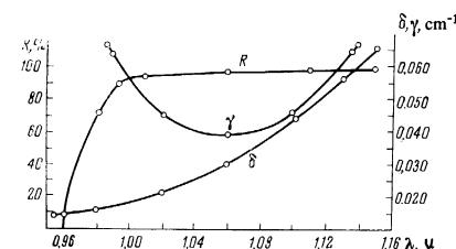
FIG. 6. Dependence of  $R$ ,  $\delta$ , and  $\gamma$  on the wavelength.  $\delta$  — is damping decrement of the KDP crystal and  $\gamma$  is a quantity proportional to  $\sqrt{P_p^{thr}}$  [1].
