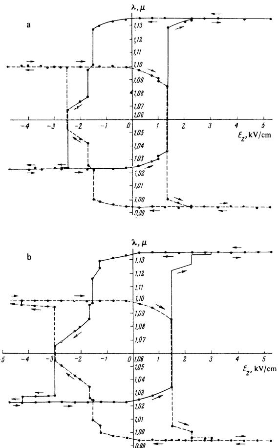
FIG. 9. Wavelength tuning of the parametric laser for two consecutive polarization reversal cycles of the crystal at  $T < T_c$  ( $T = 109^\circ\text{K}$ ). a - 1st cycle; b - 2nd cycle. Arrows indicate the cycling direction.
