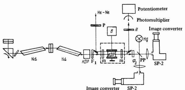
FIG. 3. Diagram of the experimental setup.  $F_1$  — liquid filter;  $F_2$  — KS-10 filter;  $B$  — high-voltage supply;  $PP$  — plane-parallel glass plate;  $P$  — polarizer;  $A$  — analyzer.
