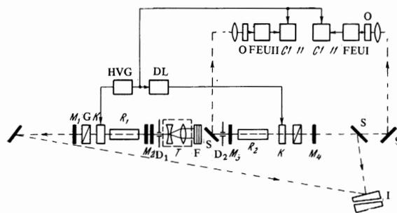
FIG. 1. Diagram of the experimental setup.  $M_1, M_4$  – mirrors with 98% reflectivity;  $M_2$  – resonance mirror;  $M_3$  – mirror with 30% reflectivity;  $R_1, R_2$  – ruby crystals;  $G$  – polarizer;  $K$  – Pockels cell;  $D_1, D_2$  – diaphragms with 0.8 mm diameter;  $T$  – telescope;  $F$  – neutral filters;  $S$  – semitransparent mirror;  $I$  – Fabry-Perot etalon;  $O$  – opal glass;  $HVG$  – high-voltage pulse generator;  $DL$  – delay line.
