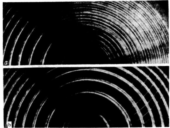
FIG. 3. Interference pattern of emission. Left –  $R_1$  ruby; right –  $R_2$  ruby; a – for  $\Delta W = 0$ ; b – for  $\Delta W = 10^{-4}$  J.
