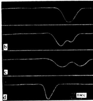
FIG. 2. Oscilloscope traces of  $R_2$  ruby emission pulses. a – c – for  $\Delta W = 0$ ; d – for  $\Delta W = 10^{-4}$  J.
