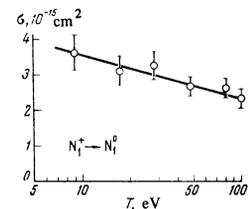
FIG. 5. Cross section for resonant charge transfer from nitrogen ions to nitrogen atoms as a function of the interaction energy.
