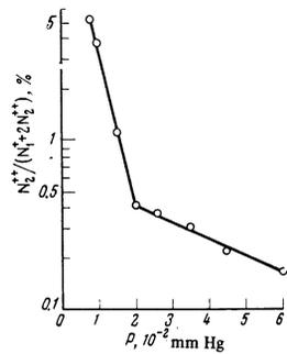
FIG. 3. Percentage of  $N_2^{++}$  in the primary ion beam as a function of nitrogen pressure in the gas discharge chamber of the ion source (having 60-V discharge voltage).
