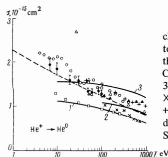
FIG. 2. Cross section for resonant charge transfer from helium ions to helium atoms as a function of the collision interaction energy. Curve 1—from [7], 2—from [8], 3—from [9]; data of □—[10], ×—[11], ▲—[12], ○—[13], △—[14], +—[15], ●—present work. The dashed curve is that calculated by Smirnov and Chibisov.<sup>[6]</sup>
