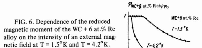
FIG. 6. Dependence of the reduced magnetic moment of the WC + 6 at.% Re alloy on the intensity of an external magnetic field at  $T = 1.5^\circ\text{K}$  and  $T = 4.2^\circ\text{K}$ .
