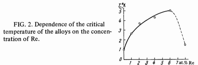
FIG. 2. Dependence of the critical temperature of the alloys on the concentration of Re.
