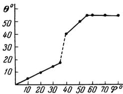
FIG. 6. Dependence of the angle  $\theta$  between  $M_S$  and  $[100]$  on the angle  $\varphi$  between  $H$  and  $[100]$  at  $H = 21.7$  kOe and  $T = 4.2^\circ\text{K}$ .
