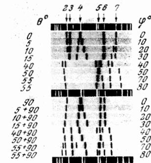
FIG. 5. Absorption spectrum of ErIG in polarized light. The angle  $\theta$  between the vector  $E$  of linearly polarized light and the  $[100]$  direction corresponds to maximum intensity of the polarized absorption bands.  $0^\circ \leq \varphi \leq 80^\circ$ ;  $H = 21.7$  kOe;  $T = 4.2^\circ\text{K}$ .
