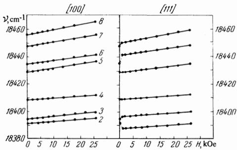
FIG. 3. Absorption band frequencies for the  ${}^4I_{15/2} \rightarrow {}^4S_{3/2}$  transition in ErIG vs. external magnetic field strength, for  $H \parallel [100]$  and  $H \parallel [111]$ , at  $4.2^\circ\text{K}$ .
