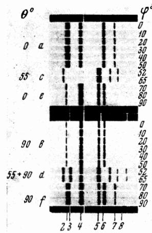
FIG. 4. Absorption spectrum of ErIG in polarized light. The angle  $\theta$  between the vector  $E$  of linearly polarized light and the  $[100]$  direction corresponds to maximum intensity of the polarized absorption bands.  $0^\circ \leq \varphi \leq 90^\circ$ ;  $H = 1.05$  kOe;  $T = 4.2^\circ\text{K}$ .
