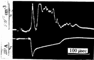
FIG. 5. Oscilloscope of plasma density and discharge current.  $H_0 = 1000$  Oe,  $C_{dir} = 2 \mu F$ ,  $U_{dir} = 2$  kV,  $L_{ch} = 100 \mu H$ , working gas — hydrogen. Mirror coils 1 and 2 connected.
