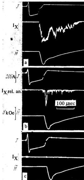
FIG. 8. Oscilloscope traces of discharge current  $J$ , of pulsed magnetic compression field  $H$ , and x-ray bremsstrahlung intensity  $I_X$  from the trap: a — both coils 1 and 2 connected, b — coil 2 connected, c — coils 1 and 2 disconnected (homogeneous magnetic field).  $H_0 = 800$  Oe,  $C_{dir} = 2 \mu F$ ,  $U_{dir} = 2.5$  kV, working gas — hydrogen.
