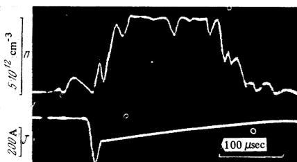
FIG. 2. Oscilloscope traces of plasma density and discharge current.  $H_0 = 1000 \text{ Oe}$ ,  $C_{\text{dir}} = 2 \mu\text{F}$ ,  $U_{\text{dir}} = 2 \text{ kV}$ ,  $L_{\text{ch}} = 100 \mu\text{H}$ , working gas – hydrogen, mirror coils 1 and 2 connected.
