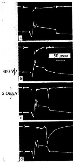
FIG. 7. Oscillograms of magnetic field in plasma (upper curves) and discharge current (lower curves): a — coils 1 and 2 disconnected (homogeneous field), b — only coil 1 connected, c — only coil 2 connected, d — both coils 1 and 2 connected.  $H_0 = 1000$  Oe,  $C_{\text{dir}} = 2 \mu\text{F}$ ,  $U_{\text{dir}} = 2.5$  kV,  $L_{\text{ch}} = 100 \mu\text{H}$ , working gas — hydrogen.
