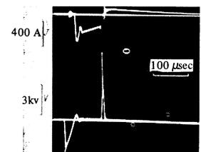
FIG. 4. Current and discharge-voltage oscilloscope traces.  $H_0 = 200 \text{ Oe}$ ,  $C_{\text{dir}} = 2 \mu\text{F}$ ,  $U_{\text{dir}} = 3 \text{ kV}$ ,  $L_{\text{ch}} = 100 \mu\text{H}$ , working gas – hydrogen, homogeneous magnetic field.
