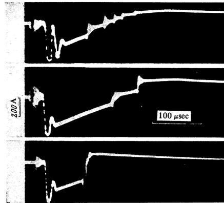
FIG. 3. Typical oscilloscope traces of the discharge current in the "current interruption" regime.
