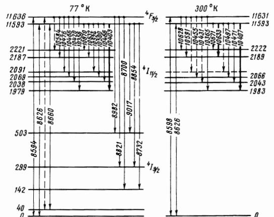
FIG. 6. Crystalline splitting of the  ${}^4F_{3/2}$ ,  ${}^4I_{11/2}$ , and  ${}^4I_{9/2}$  terms of the  $\text{LaF}_3\text{-Nd}^{3+}$  crystal. Level positions are in  $\text{cm}^{-1}$  and the transitions in Å. Stimulated transitions are denoted by heavy arrows.
