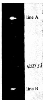
FIG. 5. Generation spectrum of  $\text{LaF}_3\text{-Nd}^{3+}$  crystal at 300°K. The position of the reference third-order iron lines is shown.
