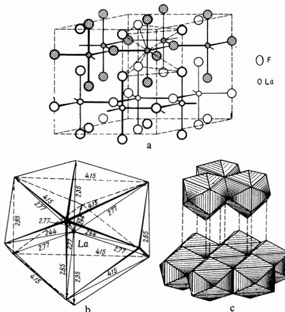
FIG. 1. Structure of the  $\text{LaF}_3$  crystal. (a) – stratified pattern of crystalline structure; (b) – eleven-vertex envelope of the  $\text{La}^{3+}$  ion; (c) – packing of polyhedra in the  $\text{LaF}_3$  crystal.
