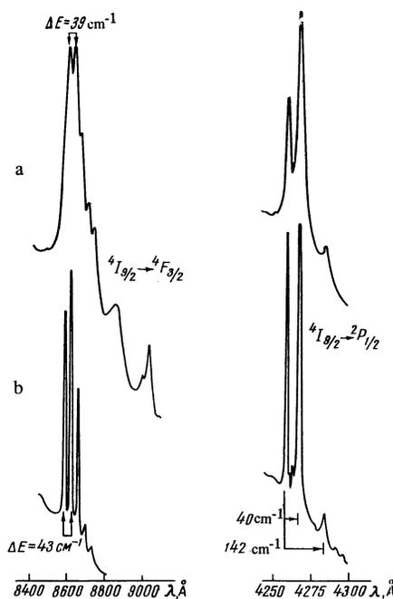
FIG. 3. Absorption spectrum of LaF<sub>3</sub>-Nd<sup>3+</sup> crystal corresponding to transitions <sup>4</sup>I<sub>9/2</sub> → <sup>4</sup>F<sub>3/2</sub> and <sup>4</sup>I<sub>9/2</sub> → <sup>2</sup>P<sub>1/2</sub>: (a) - at 300°K, and (b) - at 77°K.
