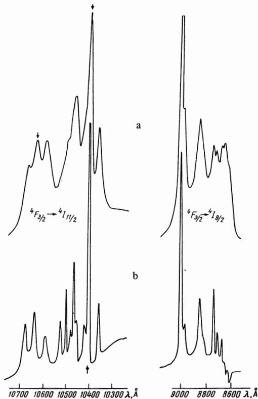
FIG. 4. Luminescence spectra of  $\text{LaF}_3\text{-Nd}^{3+}$  crystal, transitions  ${}^4F_{3/2} \rightarrow {}^4I_{11/2}$  and  ${}^4F_{3/2} \rightarrow {}^4I_{9/2}$ : (a) - at 300°K, and (b) - at 77°K.
