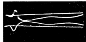
FIG. 5. Oscillograms of signals from a cylindrical charge with horizontal axis exploded by flame ignition at one end. Upper sweep-signal from antenna forming 180^\circ with initiation direction ( R = 10 m); lower sweep-antenna forming 45^\circ angle ( R = 8 m). Charge mass 1.3 kg; H/d = 4.6 ; height above surface of earth 3 m; \Delta t = 1.0 millisecc.
