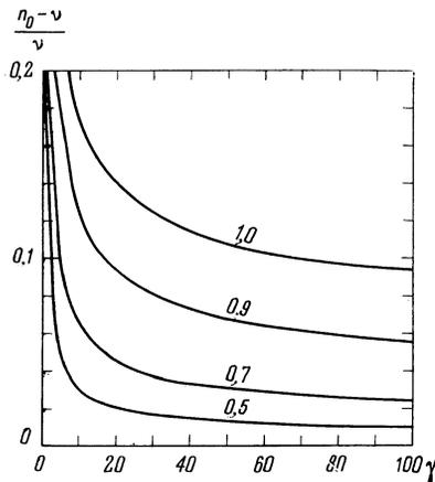
FIG. 1.  $(n_0 - \nu)/\nu$  as a function of  $\gamma$ . The numbers of the curves indicate the values of the ellipticity  $\varepsilon$  of the light.
