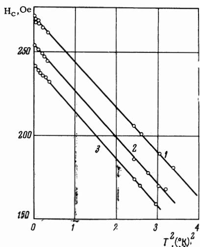
FIG. 4. Critical field curves of indium illustrating the determination of  $H_{0c}$ : 1 -  $p = 1800$  atm, 2 -  $p = 6600$  atm, 3 -  $p = 9600$  atm.
