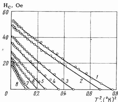
FIG. 8. Critical field curves of zinc at various pressures: 1 -  $p = 0$ , 2 -  $p = 3000$  atm, 3 -  $7300$  atm, 4 -  $p = 11,800$  atm, 5 -  $p = 15,600$  atm, 6 -  $p = 19,800$  atm, 7 -  $p = 23,900$  atm, 8 -  $p = 26,200$  atm.
