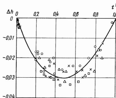
FIG. 5. The deviation  $[\Delta h = h - (1 - t^2)]$  of the critical-field curves from a parabola in tin at various pressures:  $\circ - p = 1400$  atm,  $\times - p = 20,000$  atm,  $\square - p = 6600$  atm,  $\Delta - p = 11,900$  atm.
