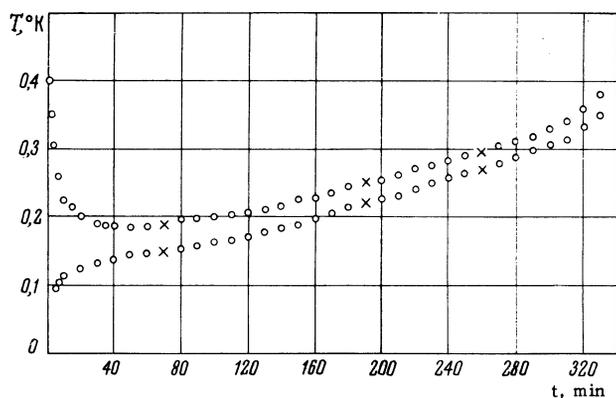
FIG. 1. Curves of the establishment of thermal equilibrium. The lower curve refers to the working salt with a ratio of axes 4 : 1 whose temperature practically coincides with the thermodynamic temperature; the upper curve refers to the salt located in the booster. x — points obtained on converting the temperature of the salt in the booster to the thermodynamic temperature.
