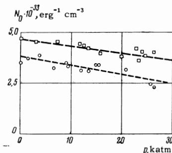
FIG. 9. Curve of the pressure dependence of the density of electron states  $N_0$  in cadmium and zinc:  $\circ$  - cadmium,  $\square$  - zinc.
