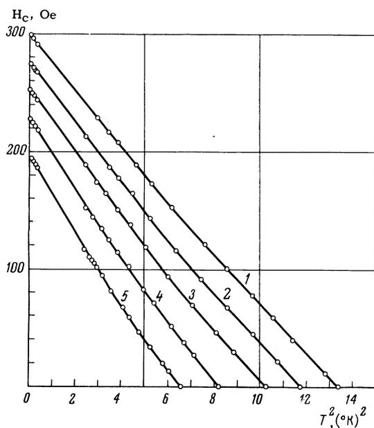
FIG. 2. Critical field curves of tin at various pressures: 1 —  $p = 1400$  atm, 2 —  $p = 6600$  atm, 3 —  $p = 11,900$  atm, 4 —  $p = 20,000$  atm, 5 —  $p = 31,600$  atm.
