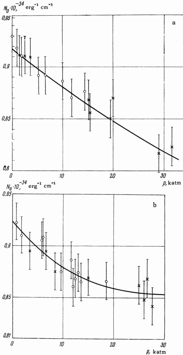
FIG. 7. Pressure dependence of the density of electron states  $N_0$ : a - in tin, b - in indium,  $\times$  - points obtained with a piston of VK-3,  $\circ$  - points obtained with a bronze piston.
