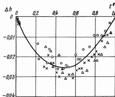
FIG. 6. The deviation of the critical-field curves from a parabola in indium at various pressures:  $\times - p = 6600$  atm,  $\circ - p = 1800$  atm,  $\Delta - p = 18,000$ .
