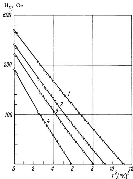
FIG. 3. Critical field curves of indium at various pressures: 1 —  $p = 1800$ , 2 —  $p = 9600$  atm, 3 —  $p = 15,000$  atm, 4 —  $p = 25,000$  atm.
