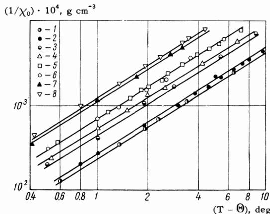
FIG. 6. Dependence of  $1/\chi_0$  on  $(T - \Theta)$  on a logarithmic scale for all ferrites investigated: 1, Y; 2, Sm; 3, Eu; 4, Er; 5, Gd; 6, Dy; 7, Ho; 8, Tb.
