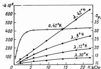
FIG. 3. Dependence of the magnetostriction and the magnetization of holmium iron garnet in the [111] direction on the magnetic field.
