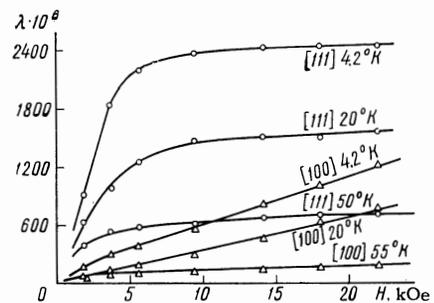
FIG. 1. Isotherms of magnetostriction of single-crystal terbium iron garnet in the [100] and [111] directions.
