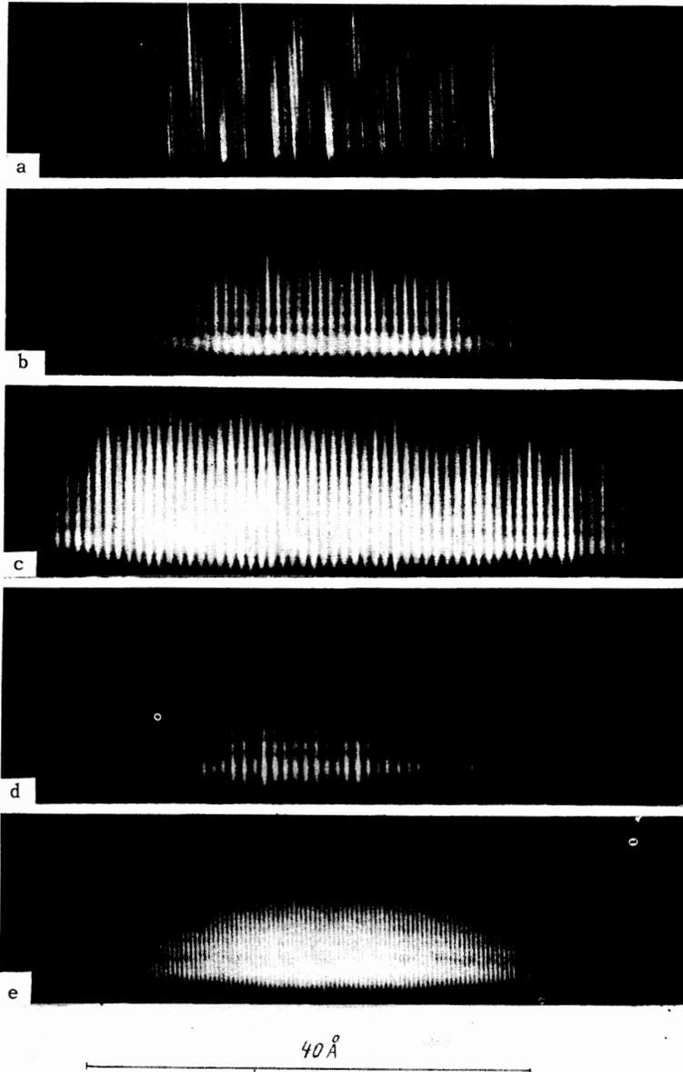
FIG. 2. Emission spectra of neodymium glass laser. a – fixed rod; b – e – moving rod; c – increased pumping; d – increased resonator length, e – identical thick substrates for mirrors,  $d_{1,2} = 8$  mm.
