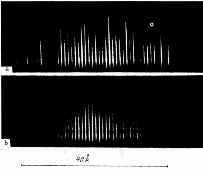
FIG. 3. Laser emission spectra obtained with identical thin mirror substrates. a - fixed rod; b - moving rod.
