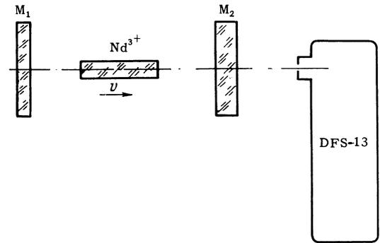
FIG. 1. Experimental setup.  $\text{Nd}^{3+}$  - glass rod doped with  $\text{Nd}^{3+}$ ;  $M_1$  and  $M_2$  - plane dielectric mirrors, DFS-13 - spectrograph.
