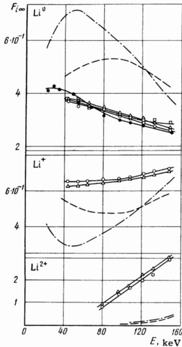
FIG. 5. Equilibrium distribution of charges in a beam of Li ions as a function of energy:  $\Delta$  – in magnesium film,  $\circ$  – in cadmium film,  $\square$  – in silver film,  $\bullet$  – in celluloid film; dot-dash curve – in magnesium vapor according to our previous work, [14] dashed curve – in cadmium vapor according to our previous work [14] (for  $\text{Li}^{2+}$  the ordinate scale is multiplied by  $1 \times 10^{-2}$ ).
