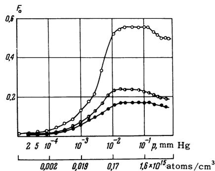
FIG. 1. Neutral component of the particle beam as a function of cadmium vapor pressure:  $\circ$  – Li ions, 96 keV;  $\bullet$  – Na ions, 96 keV;  $\bullet$  – K ions, 80 keV.
