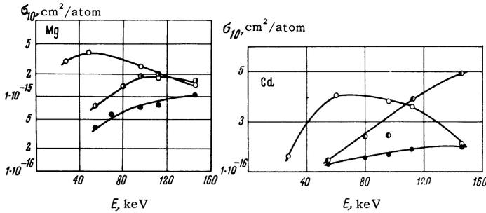
FIG. 2. Cross sections for electron capture by Li, Na, and K ions in magnesium and cadmium vapor as a function of energy:  $\circ$  -  $\text{Li}^+$ ,  $\bullet$  -  $\text{Na}^+$ ,  $\bullet$  -  $\text{K}^+$ .
