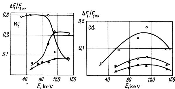
FIG. 3. Relative increase in the singly charged component as a function of ion energy in magnesium and cadmium vapors:  $\circ$  - Li ions,  $\bullet$  - Na ions,  $\bullet$  - K ions.
