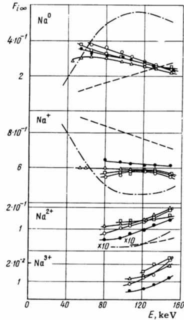
FIG. 6. Equilibrium distributions of charges in a beam of Na ions as a function of energy:  $\Delta$  – in magnesium film,  $\circ$  – in cadmium film,  $\square$  – in silver film,  $\bullet$  – in celluloid film; dot-dash curve – in magnesium vapor according to our previous work, [14] dashed curve – in cadmium vapor according to our previous work. [14]
