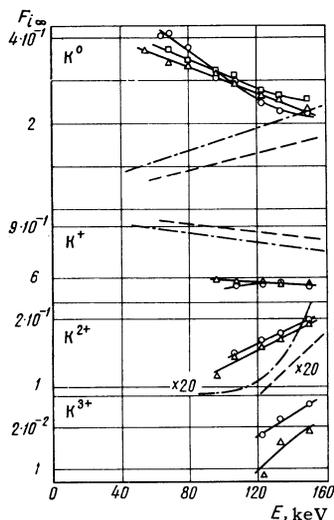
FIG. 7. Equilibrium charge distributions in a beam of K ions as a function of energy:  $\Delta$  – in magnesium film,  $O$  – in cadmium film,  $\square$  – in silver film; dot-dash curve – in magnesium vapor according to our previous work, [<sup>14</sup>] dashed curve – in cadmium vapor according to our previous work. [<sup>14</sup>]
