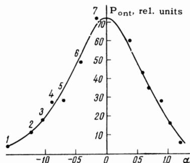
FIG. 2. Emission power as a function of spherical mirror angle for a laser with a plane + sphere resonator ( $R = 2m$ ).
