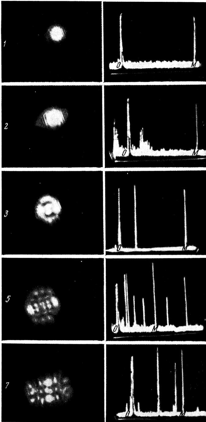
FIG. 3. Variation in emission field structure and beats spectrum due to spherical-mirror ( $R = 2$  m) rotation. 0 – zero frequency, M – marker for 2 MHz.
