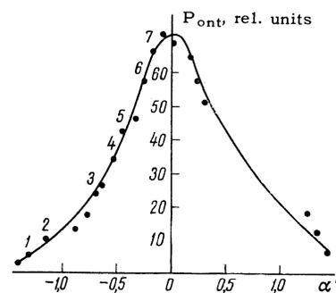
FIG. 4. Emission power as a function of spherical mirror angle ( $R = 4$  m).
