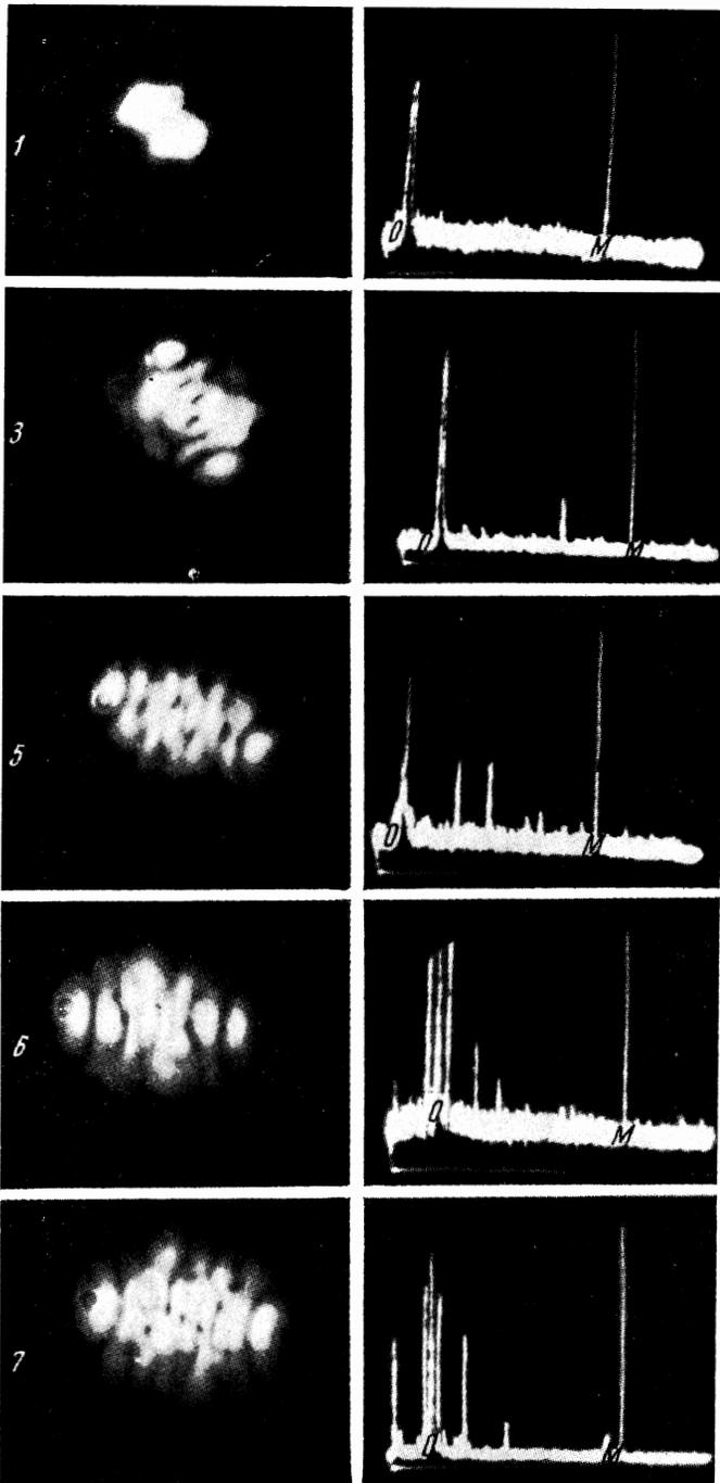
FIG. 5. Variation in emission field structure and beats spectrum due to spherical-mirror ( $R = 4$  m) rotation. 0 – zero frequency, M – marker for 2 MHz.
