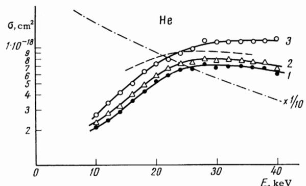
FIG. 4. Excitation cross sections resulting from proton-helium charge exchange vs. proton energy: 1—Cross section for  $L_\beta$  emission in zero field, 2—for excitation of the  $3p$  state, 3— $L_\beta$  emission in a field. The dashed curve pertains to  $3p$  excitation data in<sup>[6]</sup>; the dot-dash curve pertains to  $3p$  excitation data in<sup>[5]</sup>.
