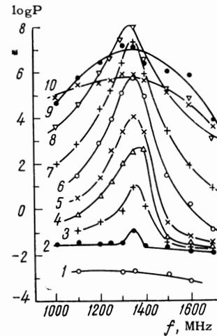
FIG. 2. Oscillation spectrum at different distances from the gun (mm): 1-30, 2-60, 3-80, 4-100, 5-120, 6-140, 7-160, 8-200, 9-230, 10-275. The same conditions as in Fig. 1.
