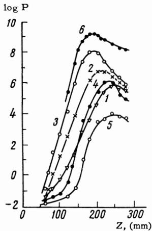
FIG. 1. Spatial distribution of the oscillation power along the tube. Frequencies (MHz): 1-1100, 2-1250, 3-1350, 4-1500, 5-1700, 6-integral oscillation power.  $i_{beam} = 16.5$  mA,  $U = 1140$  V,  $H = 190$  Oe.
