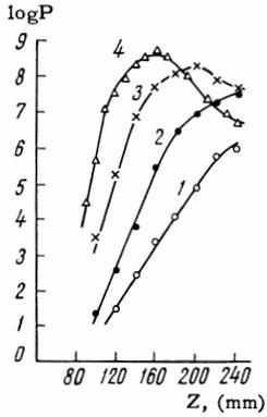
FIG. 3. Spatial distribution of the oscillation power along the tube at different beam currents.  $f = 1300$  MHz;  $U = 1200$  V. 1- $i = 10$  mA,  $H = 197$  Oe; 2- $i = 12$  mA,  $H = 190$  Oe; 3- $i = 16.5$  mA,  $H = 185$  Oe; 4- $i = 22$  mA,  $H = 175$  Oe.
