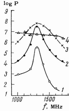
FIG. 4. Oscillation spectra measured near the collector ( $z = 240$  mm) at different values of the beam current. The conditions are the same for Fig. 3.
