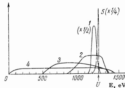
FIG. 5. Normalized beam-electron energy distribution functions measured at a distance 260 mm from the gun at different values of the beam ( $i_s = 2$  mA). The conditions are the same as in Figs. 3 and 4.
