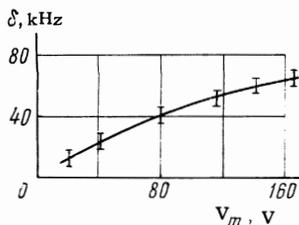
FIG. 4. Laser synchronization region vs. modulating voltage.
