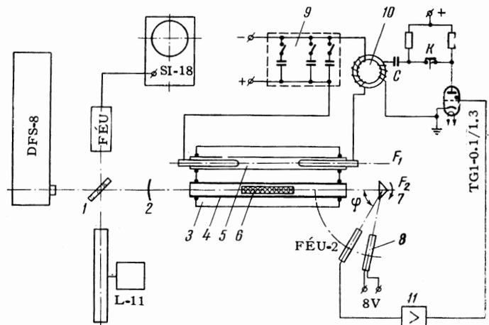
FIG. 1. Block diagram of apparatus: 1) plane-parallel glass plate; 2) spherical dielectric mirror; 3) cylindrical illumination chamber of elliptical cross section; 4) tubular filter of BS or ZhS-17 glass; 5) IFP-800 xenon pulse-discharge lamp; 6) working crystal; 7)  $90^\circ$  total-internal-reflection glass prism; 8) light source; 9) bank of IM-5-150 pulse-discharge capacitors; 10) hf pulse transformer; 11) pulse amplifier.
