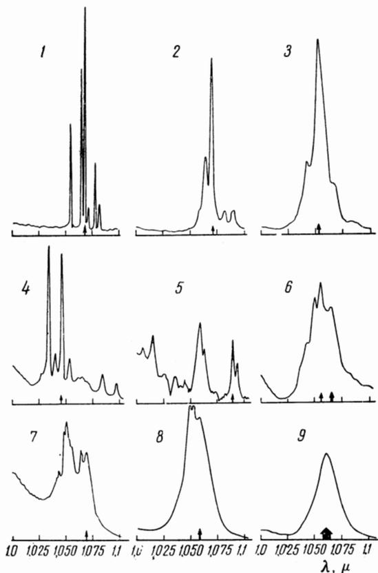
FIG. 4. Luminescence spectra of the  ${}^4F_{3/2} \rightarrow {}^4I_{11/2}$  transition of the  $Nd^{3+}$  ion at  $300^\circ K$  in crystals: 1)  $Y_3Al_5O_{12}$ ; 2)  $CaWO_4$ ; 3)  $BaF_2-LaF_3$ ; 4)  $CaF_2$  type I; 5)  $CaF_2$  type II; 6)  $CaF_2-YF_3$ ; 7)  $CaF_2-CeF_3$ ; 8)  $SrF_2-LaF_3$ ; 9) KGSS-7 glass. Arrows indicate emission lines under free generation conditions and their relative widths.
