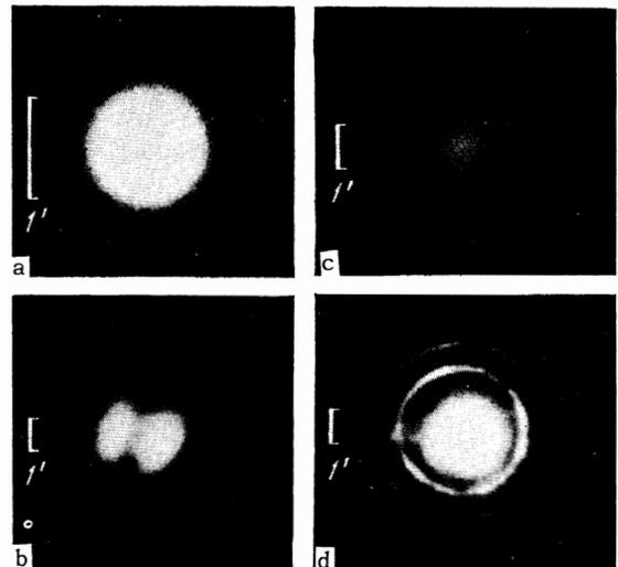
FIG. 1. Photographs of the angular distribution of laser emission. a – neodymium glass; red length  $l = 4.0$  cm, diameter  $D = 0.8$  cm, resonator length  $L = 100$  cm, excess pump power  $n = 20$ . b, c, d –  $\text{CaF}_2:\text{Sm}^{2+}$ ;  $l = 4$  cm,  $D = 0.5$  cm. b –  $L = 100$  cm,  $n \approx 1$ ,  $\text{TEM}_{00}$  mode. c –  $L = 60$  cm,  $n \approx 1$ ,  $\text{TEM}_{01}$  mode. d –  $L = 45$  cm,  $n = 16$ .
