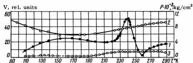
FIG. 3. Temperature dependence of the induced emf at an initial pressure of 9400 kg/cm<sup>2</sup>. Curve 1—measuring coil with sample; curve 3—without sample. Curve 2—pressure variation in the chamber as the temperature is lowered.
