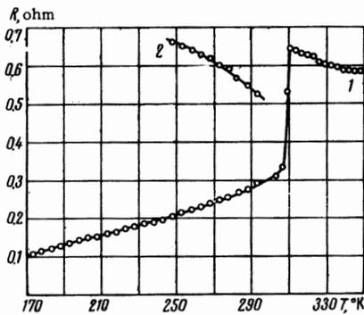
FIG. 6. Temperature dependence of the electrical resistance of MnAs. Curve 1—at atmospheric pressure; curve 2—at  $P = 8000 \text{ kg/cm}^2$ .
