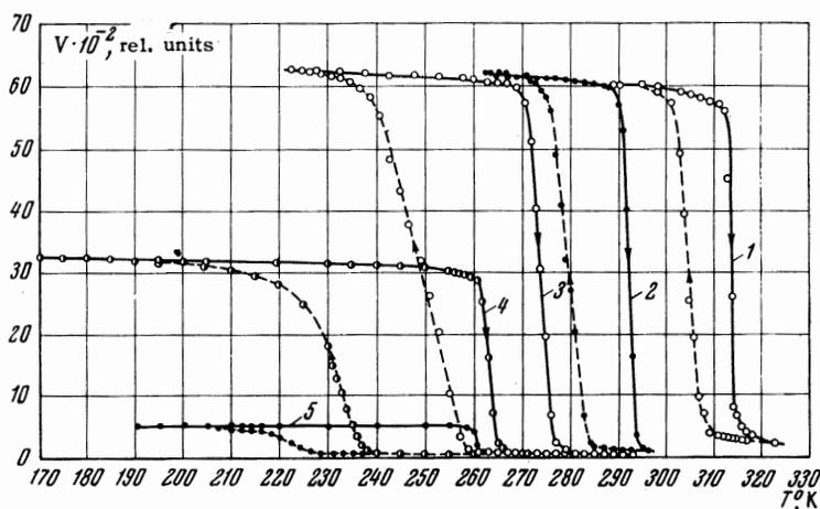
FIG. 1. Temperature dependence of the emf induced in the measuring coil (in relative units) at various pressures: 1 – atmospheric pressure; 2 –  $P = 1400 \text{ kg/cm}^2$ ; 3 –  $P = 2350 \text{ kg/cm}^2$ ; 4 –  $P = 2970 \text{ kg/cm}^2$ ; 5 –  $P = 4000 \text{ kg/cm}^2$ . The solid curves were obtained during warming of the sample, the dashed curves, during cooling.
