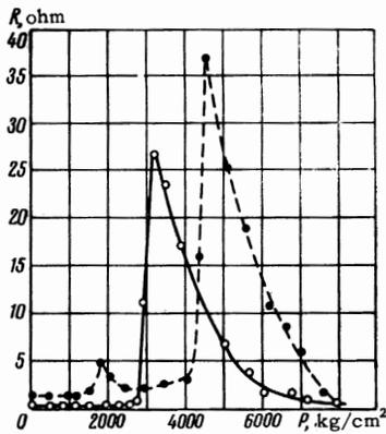
FIG. 5. Pressure dependence of the electrical resistance of MnAs, measured in the neighborhood of the transition temperature  $T_C$ .
