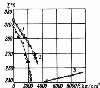
FIG. 7. Phase diagram for MnAs. Curve 1—change with pressure of the magnetic transformation temperature  $\Theta_1$ ; 2—change of the transition temperature  $T_C$ ; 3—change of the Néel point of the high-pressure phase. Dashed curve obtained during sample cooling.  $\circ$ —points obtained by magnetic measurements,  $\bullet$ —by electrical measurements.
