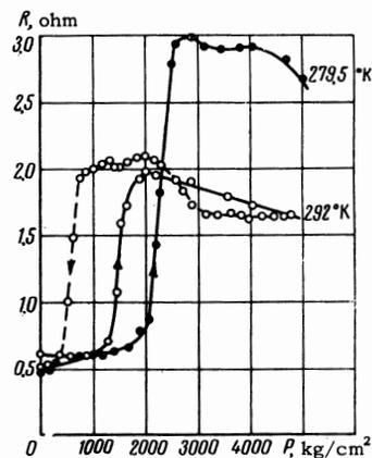
FIG. 4. Pressure dependence of the electrical resistance of MnAs, measured in the neighborhood of the magnetic transformation temperature  $\Theta_1$ .
