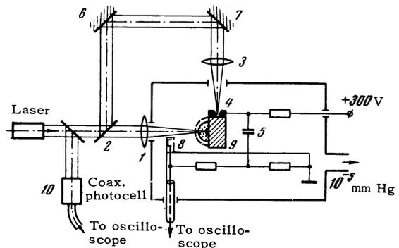
FIG. 1. Experimental setup for plotting the R-t diagram of the neutral boundary (see text for designations).
