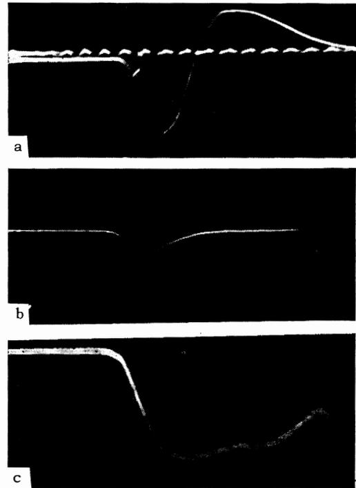
FIG. 2. Oscilloscopic traces: (a) probe signal, (b) laser emission pulse, (c) electron emission current.
