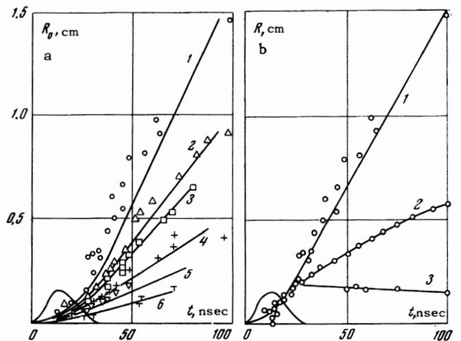
FIG. 3.  $R-t$  diagrams: (a) neutral boundary for various power values, (b) neutral boundary (curve 1), luminous edge (curve 2), and opaque region boundary (curve 3). Power output, 200 megawatts.
