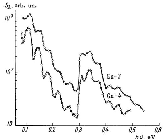
FIG. 1. Spectra of impurity photoconductivity of Ge with Ga,  $T \approx 6.5^\circ\text{K}$ ,  $E = 1.5 \text{ V/cm}$ .
