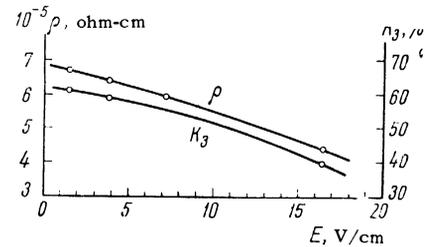
FIG. 3. Dependence of the relative depth of the third minimum on the spectrum of sample Ga-4 and of the specific resistivity of this sample on the electric field intensity ("break-down" field  $E \approx 19$  V/cm),  $T \approx 7^\circ\text{K}$ .
