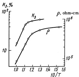
FIG. 2. Temperature dependence of the depth of the third minimum on the spectrum of the sample Ga-4 and temperature dependence of the specific resistivity of this sample under the same conditions,  $E = 1.5$  V/cm.
