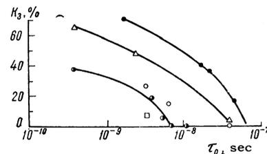
FIG. 4. Dependence of the relative depth of the third minimum on  $\tau_0$  for samples with impurities: ● — 1A Ga (0.01 eV),  $\Delta$  — 1A Zn (0.03 eV),  $\bullet$  — 1A Cu (0.04 eV),  $\circ$  — D Au (0.04 eV),  $\square$  — 1A Hg (0.087 eV);  $T \approx 8^\circ\text{K}$ ,  $E = 1.5$  V/cm.
