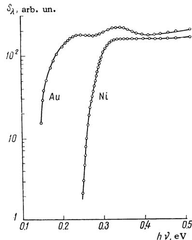
FIG. 5. Spectra of impurity photoconductivity of Ge with 1A Au and 1A Ni;  $T \approx 8^\circ\text{K}$ ,  $E = 1.5 \text{ V/cm}$ .
