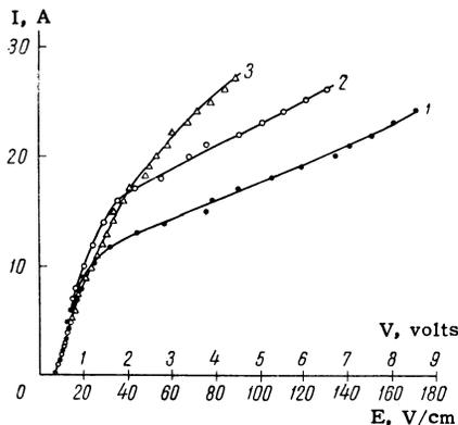
FIG. 1. Dependence of the current on the voltage in an electron-hole plasma in a longitudinal magnetic field: 1)  $H_z = 0$ ; 2)  $H_z = 200 \text{ Oe}$ ; 3)  $H_z = 350 \text{ Oe}$ ;  $T = 4.2^\circ \text{ K}$ .
