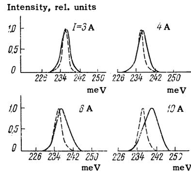
FIG. 2. Radiation spectra of a plasma for various values of the current in  $H_z = 0$  (continuous curves) and  $H_z = 350 \text{ Oe}$  (dashed curves).
