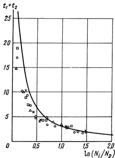
FIG. 3. Relative giant pulse length,  $t_1 + t_2$ , as a function of the population inverse coefficient.  $\circ$  - specimen 8 mm dia  $\times$  120 mm;  $\square$  - 9.3 mm dia  $\times$  108 mm;  $\times$  - 12 mm dia  $\times$  115 mm;  $\Delta$  - 15 mm dia  $\times$  120 mm.
