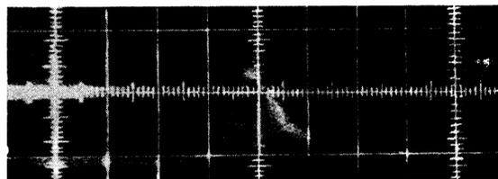
FIG. 2. Oscillographic trace of a giant pulse, for  $\tau_f = 0.4$  (specimen  $8 \times 130$  mm). Sweep 10 nsec/cm.
