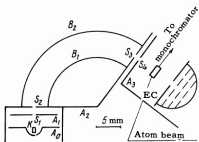
FIG. 1. Scheme of the electron monochromator.
