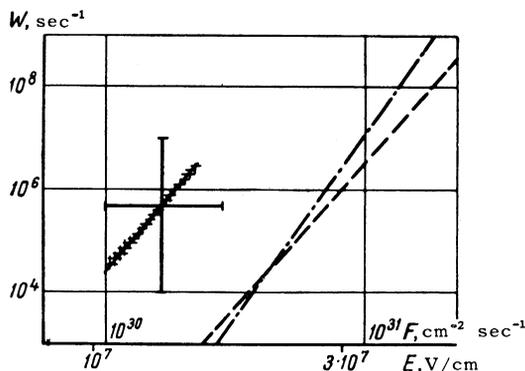
FIG. 3. Dependence of the probability of the many-photon ionization of the xenon atom on the intensity of the photon beam (the electric field intensity) for  $\hbar\omega = 1.79$  eV. The results of calculation are also given: the dashed line represents the calculations made in accordance with [1] for the six-photon process; the chain line represents the calculations made in accordance with [7] allowing for resonance levels.
