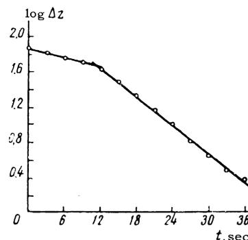
FIG. 2. Dependence  $\log \Delta z = f(t)$  for water. Angular velocity  $\omega_0 = 56.5 \text{ sec}^{-1}$ .
