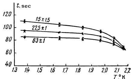
FIG. 7. Dependence of the time of penetration of the meniscus to  $3/4$  of the equilibrium depth for helium II on the temperature:  $\bullet$  -  $R = 21 \text{ mm}$ ,  $\times$  -  $R = 12.5 \text{ mm}$ ,  $+$  -  $R = 7.5 \text{ mm}$ ,  $\circ$  -  $R = 5 \text{ mm}$ . The number on the curves are the velocity on the periphery of the container;  $v = \omega_0 R$  (in  $\text{cm}/\text{sec}$ ).
