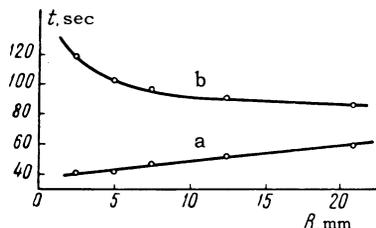
FIG. 5. Dependence of the time of the penetration of the meniscus to  $3/4$  of its equilibrium depth for helium I (curve a) and helium II (curve b) on the radius of the container;  $\omega_0 = 30 \text{ sec}^{-1}$ .
