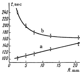
FIG. 4. Dependence of the time of complete twisting of helium I (curve a) and helium II (curve b) on the radius of the container;  $\omega_0 = 30 \text{ sec}^{-1}$ .
