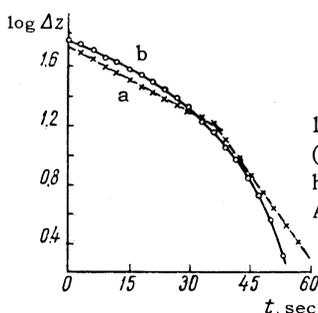
FIG. 1. Dependence of  $\log \Delta z = f(t)$  for helium I (curve a,  $T = 2.186^\circ\text{K}$ ) and helium II (curve b,  $T = 2.164^\circ\text{K}$ ). Angular velocity  $\omega_0 = 53.4 \text{ sec}^{-1}$ .
