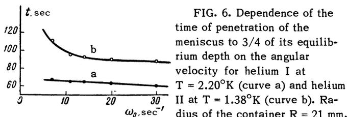
FIG. 6. Dependence of the time of penetration of the meniscus to  $3/4$  of its equilibrium depth on the angular velocity for helium I at  $T = 2.20^\circ\text{K}$  (curve a) and helium II at  $T = 1.38^\circ\text{K}$  (curve b). Radius of the container  $R = 21 \text{ mm}$ .
