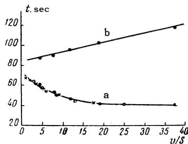
FIG. 8. Dependence of the time of penetration of the meniscus to  $3/4$  of its equilibrium depth on the ratio  $v/S \equiv \omega_0 / \pi R$  for helium I (curve a) and helium II (curve b). The different points on the curve correspond to the same diameters of the containers as in Fig. 6 ( $v$  - velocity on periphery of the container,  $S$  is the area of its cross section).
