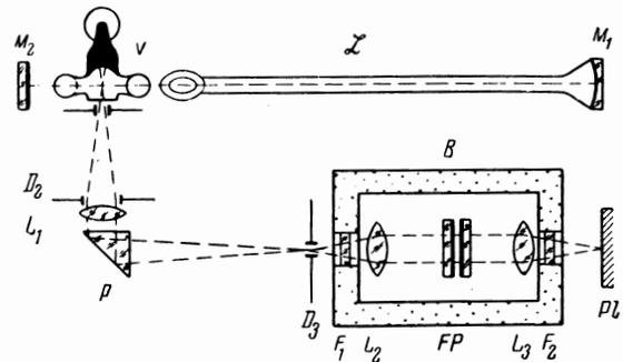
FIG. 1. The diagram of the apparatus for study of the fine structure of the Rayleigh line in liquids:  $\mathcal{L}$  = laser tube,  $M_1$  and  $M_2$  are dielectric mirrors, V = vessel with the liquid to be studied, FP – Fabry-Perot interferometer,  $L_1$ ,  $L_2$ ,  $L_3$  – objectives,  $D_1$ ,  $D_2$ ,  $D_3$  diaphragms, P – reflecting prism,  $F_1$  and  $F_2$  – light filters, Pl – film, B – isothermal chamber.
