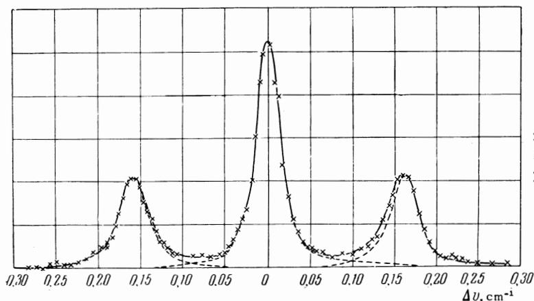
FIG. 3. Intensity distribution in components of the fine structure of the scattering lines in benzene: solid line – experimental curve, broken line – result of analysis.
