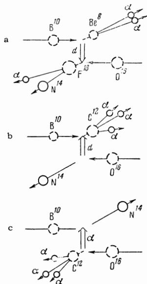
FIG. 5. Reaction mechanisms. a – deuteron capture by  $O^{16}$ , b – deuteron pickup by  $B^{10}$ , c –  $\alpha$ -particle pickup by  $B^{10}$ .
