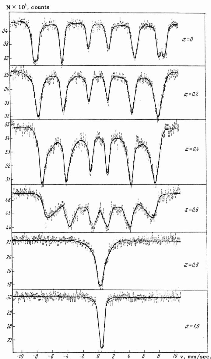
FIG. 1. Mossbauer spectra of Ni—Zn ferrites for various zinc contents ( $T = 300^\circ\text{K}$ ).
