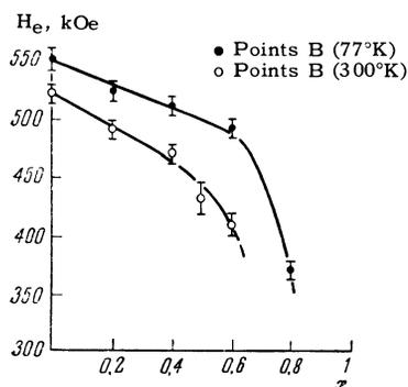
FIG. 3. Internal magnetic fields at  $\text{Fe}^{57}$  nuclei in the octahedral sublattice in the Ni-Zn series of ferrites vs. zinc content.
