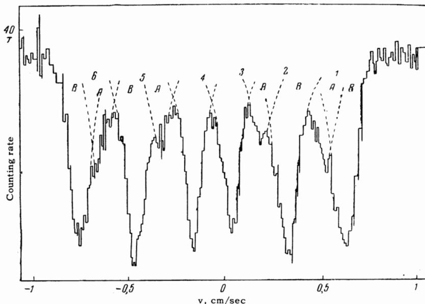
FIG. 2. Mossbauer spectrum of the Ni-Zn ferrite with  $x = 0.5$  for  $T = 300^\circ\text{K}$ .
