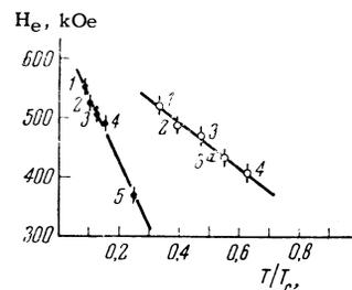
FIG. 5. Internal magnetic fields at  $\text{Fe}^{57}$  nuclei in the octahedral sublattice in the Ni-Zn series of ferrites, vs. the relative temperature  $T/T_C$ .
