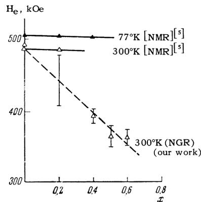
FIG. 4. Internal magnetic fields at  $\text{Fe}^{57}$  nuclei in the tetrahedral sublattice vs. zinc content  $x$ , obtained in the present work and in<sup>[5]</sup>.
