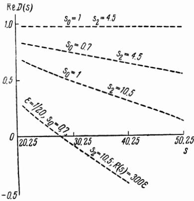
FIG. 3. Behavior of  $\text{Re}D(s)$  and its dependence on the parameters  $s_0 = s_{\text{comp}}$  and  $s_2$  ( $s_2 = 2.5$  corresponds to the contribution from  $\rho$ -exchange forces).
